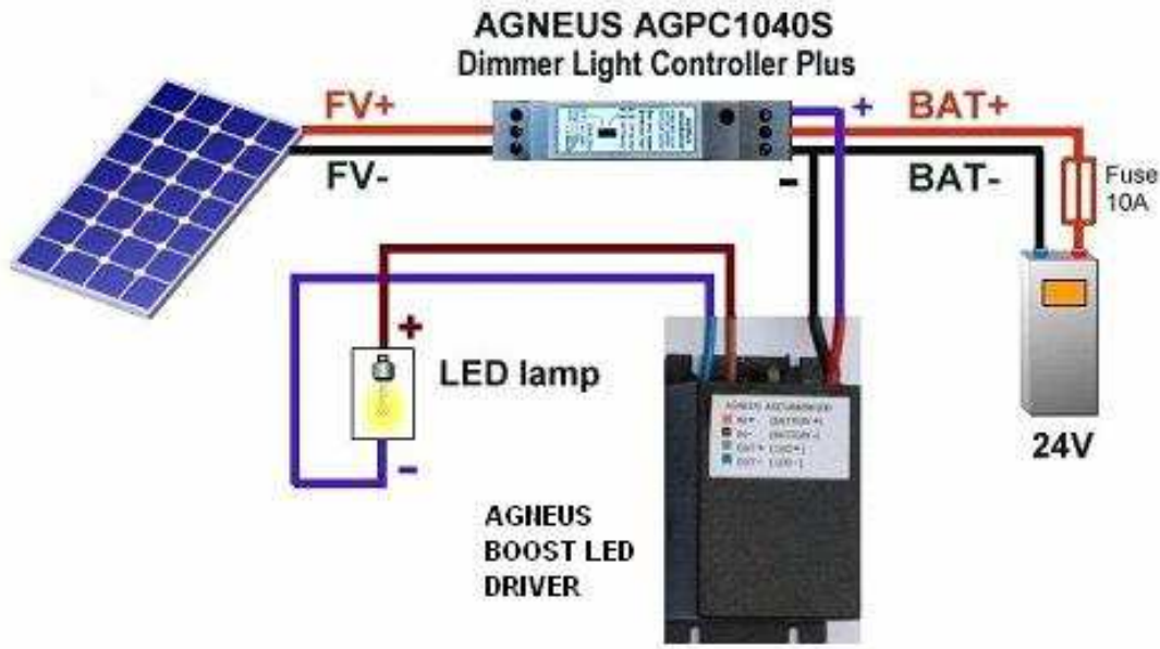
figure 1 – LED solar street lighting using AGNEUS AGCU840W48HV and AGPC1040S DLC+
